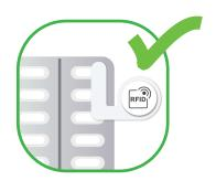
Metal can interfere with the ScripTalk Reader; use a Hang Tag for medications such as inhalers, blister packs and metal tubes.
