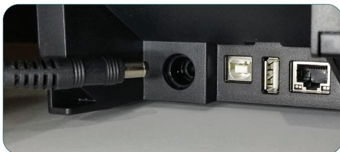
8. Connect the printer to the ScriptAbility PC with a USB cable or to the network with a Cat5 or faster Ethernet cable.
